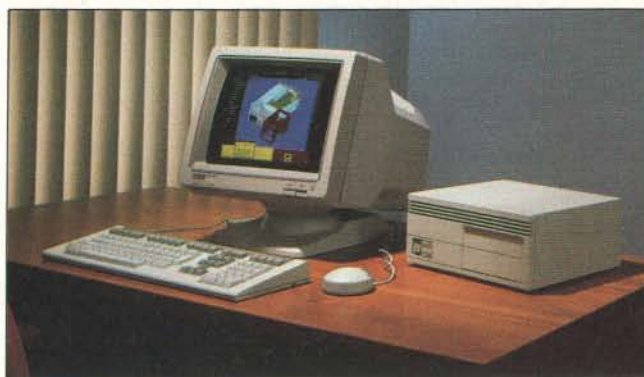
The VAXstation 2000 displays 1024-by 864-pixel color.
